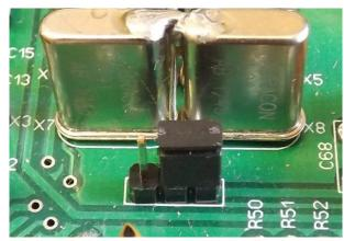
Jumper on RX IF crystal filter input
