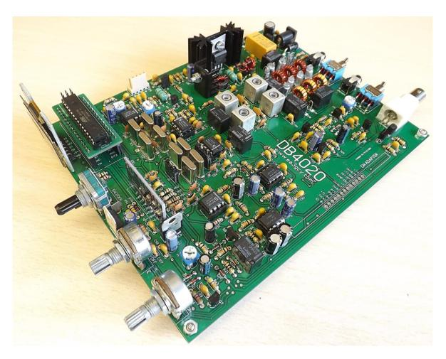
Thank you for building the **DB4020** Dual Band 40&20M SSB Transceiver kit
