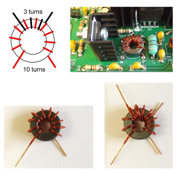
IMPORTANT: Wind the toroid exactly as shown in the images. You must pay attention to number of turns as well as to the direction of the winding.
