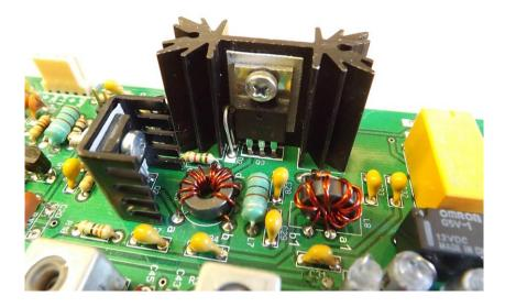
If you plan to work at maximum power and for long periods of time (at base station) it may be advisable to increase the cooling surface. You can add some system to increase the temperature dissipation, for example by an auxiliary metal surface, a mini-fan or other similar system.
