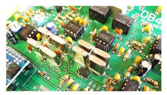
Note: With a scrap piece of wire left, you can solder the crystals housings to GND.
