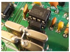
Jumper on RX IF crystal filter output
