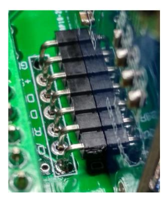
**IMPORTANT:** cut the connection terminals flush. ¡Avoid touching the front panel!
