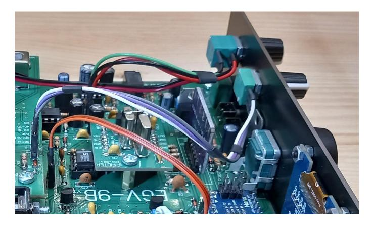
Band potentiometer wires go to "V-TUNE" on LPF/BPF module PCB. Please see how the cables are arranged in the EGV-9B assembly manual.
