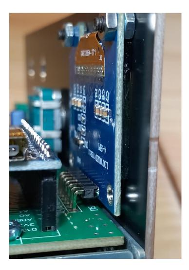
Use two M2.5 screws. It is not necessary that overtighten. Excessive tightening can damage the display. Install a nut to obtain clearance between the panel and the display (see images).
