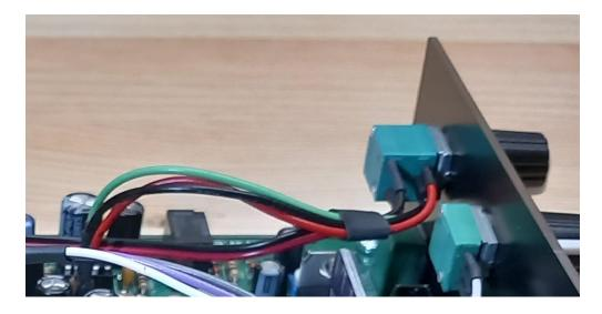
Volume potentiometer wires go to "VOLUME P4" terminals and ON/OFF switch wires to "J1" terminals (ON/OFF jumper). Please see how the cables are arranged in the EGV-9B assembly manual.
