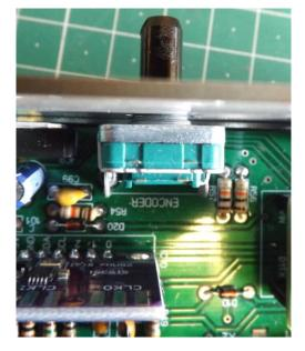
Do not screw the Encoder. This is sufficiently attached to the EGV-9B PCB.
