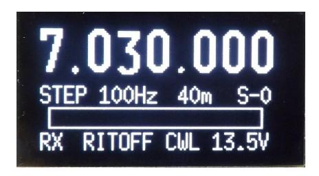
On the working dial display, you can see the tuned frequency, the current step, Band, the S-Meter, the current status (RX or TX), the RIT status (ON / OFF), the CW mode (CWL or CWU) and the supply voltage.
