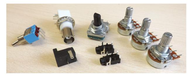
Before mounting the external connection jacks, you should cut the protrusions located at the bottom of these jacks; otherwise you will not be able to solder them in the correct position. See the image.
