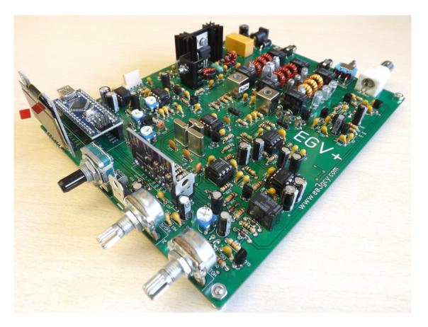
Thank you for building the EGV+v2 40, 30 and 20m QRP CW Transceiver kit
