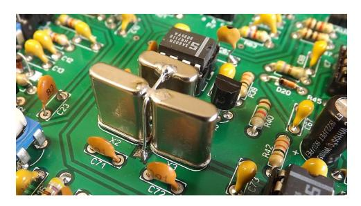
Note: With a scrap piece of wire left, you can solder the crystals housings to GND. <u>Be careful not to</u> overheat the crystals.
