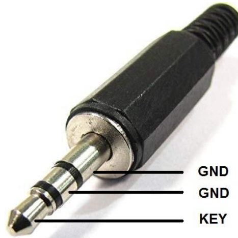
Straight keyer Jack (stereo or mono)
