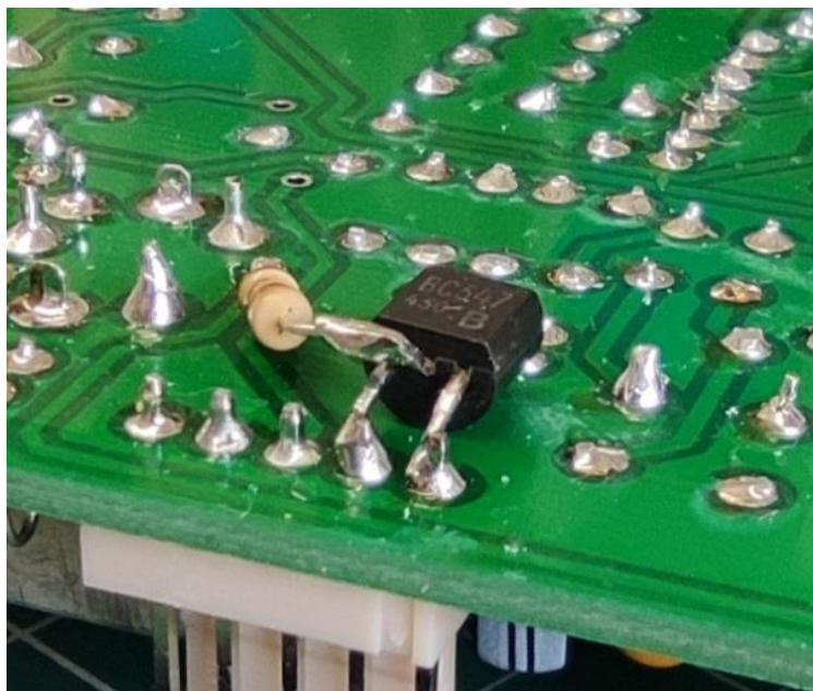
Use a 10K resistor and a BC547 transistor or equivalent.
