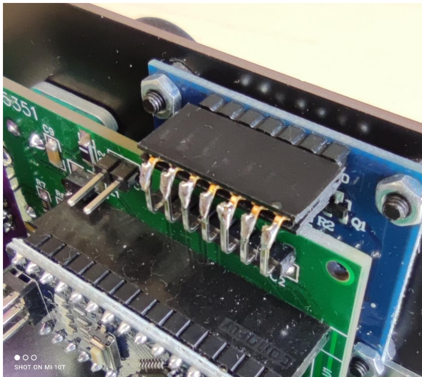
Attach the 7-pin female strip and bend its terminals as shown in the picture Then solder the terminals carefully
