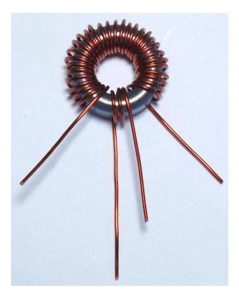
Scrape off the enamel with a cutter from the ends of the wire, in order to solder the toroid onto the board.
