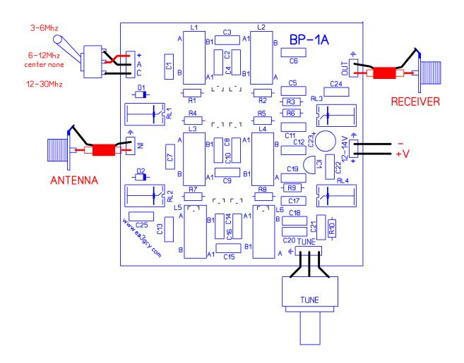
The antenna input is marked "IN" and the output to the receiver is marked "OUT" (use 50ohms coaxial cable for both connections) The 12 to 14V power supply is connected to the "12-14V" terminals.
