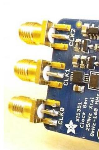
**IMPORTANT:** The outputs are not decoupled DC. If the circuit where you are going to connect the signal does not include it, you must add a 10nF or 100nF capacitor in series with the signal.
