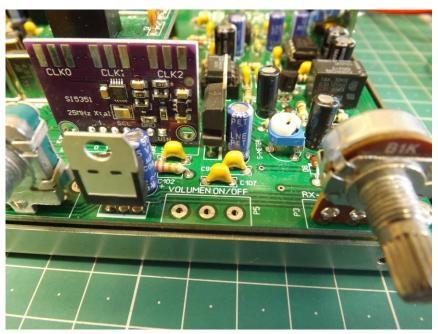
Replace the original potentiometer with the mini potentiometer with switch
