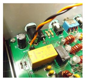
Wire the ON/OFF switch to J1 jumper
