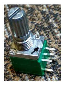
Do not screw the Encoder. This is sufficiently attached to the DB4020 PCB.
