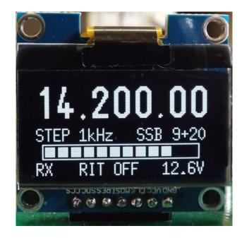
On the working dial display, you can see the tuned frequency, the current step, the mode (USB, LSB or CW), the S-Meter, the current status (RX or TX), the RIT status (ON / OFF) and the supply voltage.
