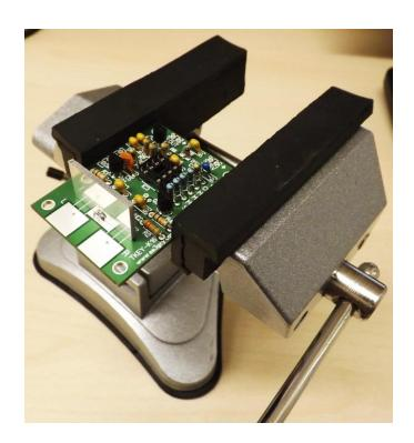
1.- With a drop of solder on each of the faces of the small piece of board that will connect to the two paddles, solder it to the main board. Obviously, it is very important that it is as vertical as possible and centered on the main circuit board.
