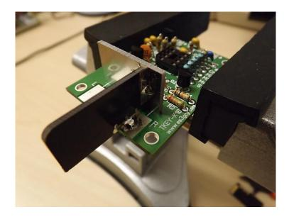
**2.-** Solder one of the paddles in its place (the two paddles are the same, because their two faces are the same). You may choose the separation between the two paddles. There are lines printed on the circuit board to help you. Decide on the position before soldering and place the two paddles so that they are centered and totally vertical with respect to the main board.
