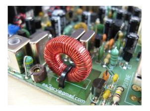
In order to make the process easier, L5 can be wound in two stages. Pass half of the wire through the toroid and wind half toroid; then, turn the toroid and wind the other half. In case of doubt about the turn count, you will be able to count them easily with a good light and a magnifying glass.
