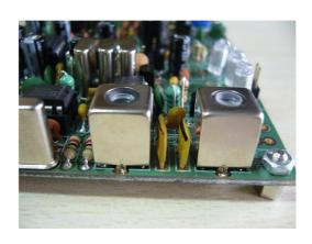
When you turn the board over the cans may fall. Fit the can in place, hold it with one hand, and turn the board over. Use the other hand for the soldering iron, and move the board towards the tin to solder the can in place. If you have someone to help out, much better!
