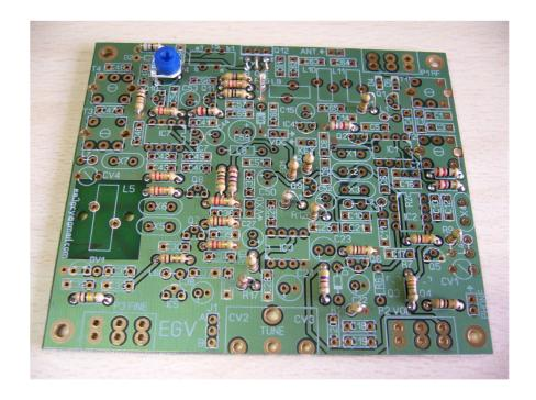
Please read the notes on soldering Poor soldering is the most common cause of a kit failing to work first time, so please take the soldering advice at heart! Once soldered cut off the excess length of the part lead as close to the joint as possible. Install all resistors from the parts list and carry on until all resistors are soldered in place.
