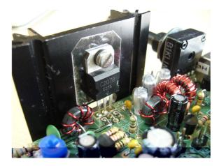
DO NOT OPERATE the transceiver without a heatsink on Q12
