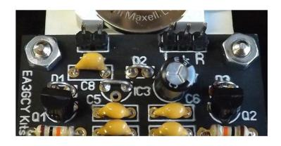
**Note:** The supplied "button" battery can deliver about 200mA and is suitable for working about 100 hours. If you are going to work a lot and everyday with the TKEY-1, it may be a good idea to use a 3.6V type LS14250 battery that can supply about 800-1200mA depending on the model).
