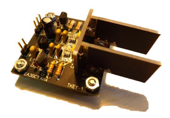
Thanks for constructing the **TKEY-1A** CW touch key
