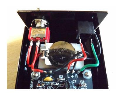
**Important**: Make sure that the entire housing (base and cover) contacts to negative pole (GND), scrape the paint around the screws (on the inside) to make electrical contact. This is very important to isolate the electronic circuit from the external RF field.
