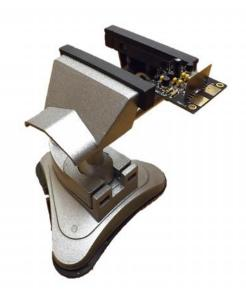
1.- With a drop of solder on each of the faces of the small piece of board that will connect to the two paddles, solder it to the main board. Obviously, it is very important that it is as vertical as possible and centered on the main circuit board.
