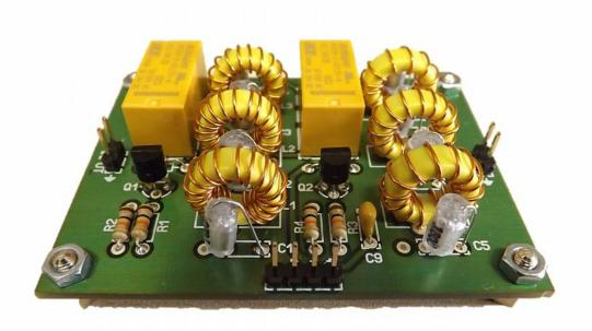
Thanks for constructing the LPF-4B low pass filter kit
