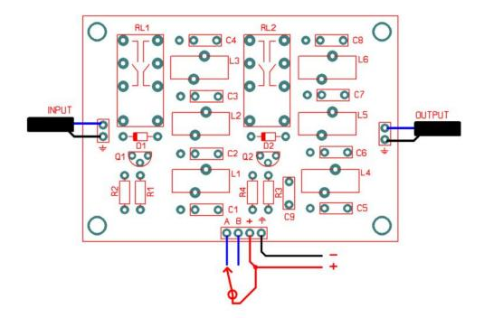
The connections of the LPF-4B are very simple. You will need a 2-position switch for the switching of the 2 filters.
