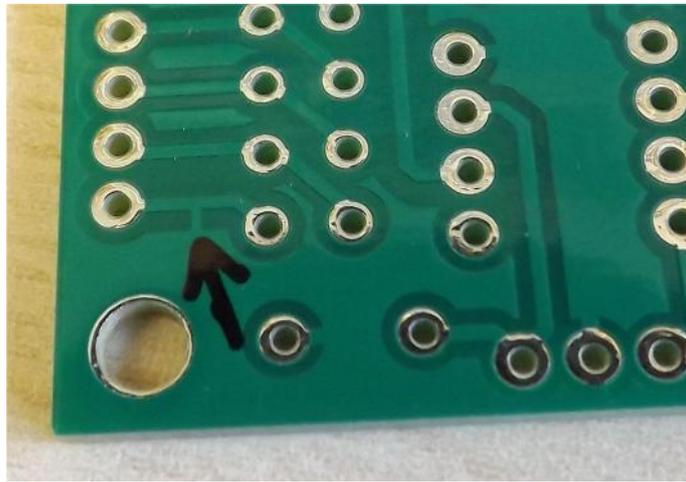
If you wish to use the speed adjustment potentiometer you must connect a 10K potentiometer to the "S" terminal and **MUST cut the circuit board track** that connects the pin with GND.
